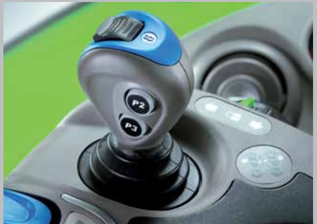
Hydraulic valves can be managed through proportional and programmable controls. The electronic Joystick can be programmed to use the front-loader and other tractor functions with the thumbwheel.
