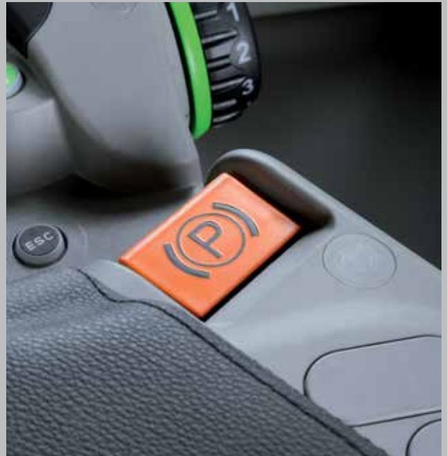
TTV models - EPB replaces the handbrake lever and is operated via an electric push-button control on the armrest console.
