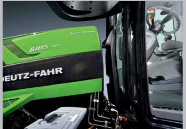
No connection between cab and engine hood - improved driver comfort.
