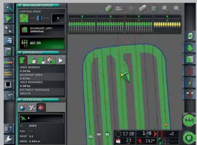
Section control/ variable rate control as standard.
