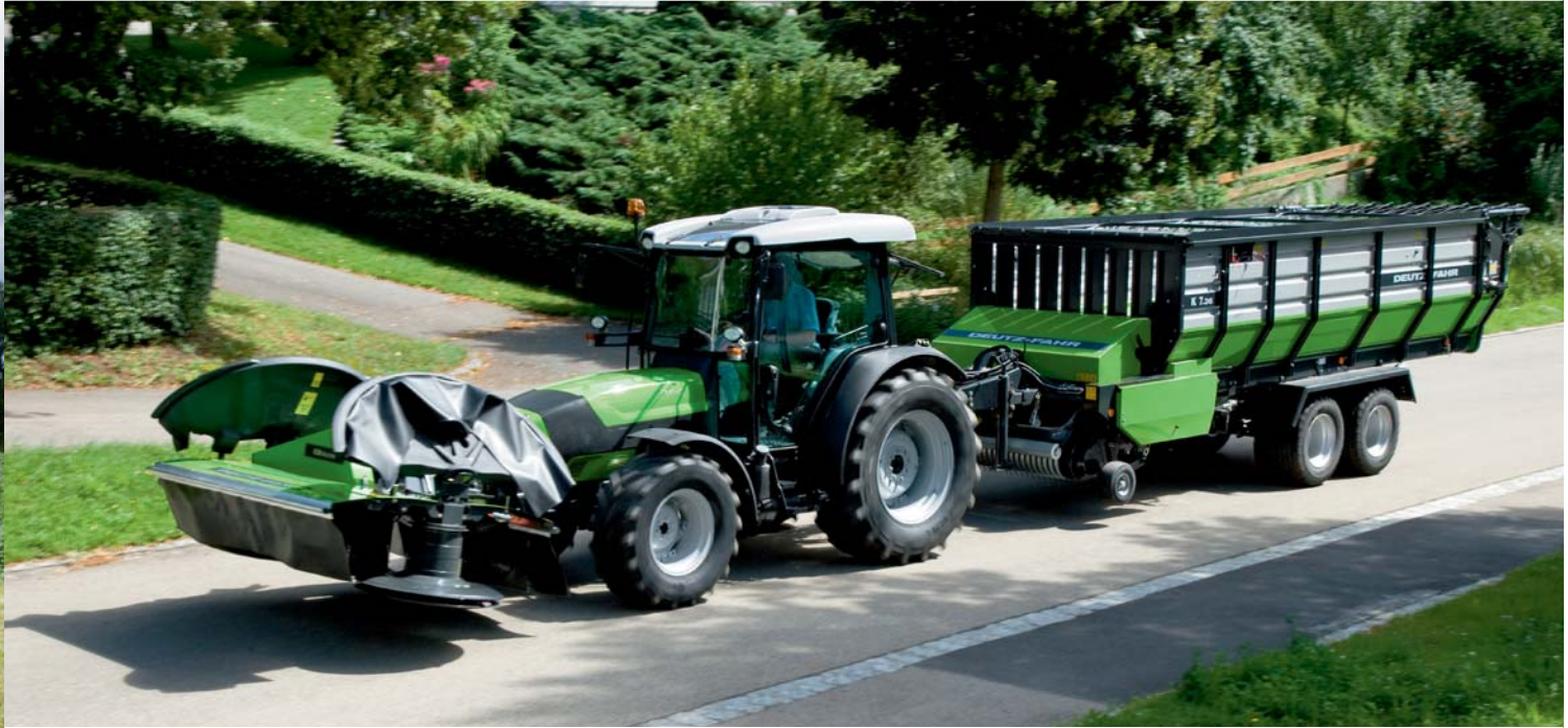
The Agroplus will fit through even low barn entrances thanks to its low external height of just 2.38 m (depending on model and tyres).
