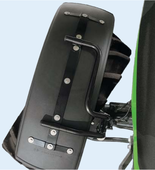
Adjustable mudguards are standard and reduce the turning circle.
