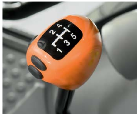
Easy shifting of the powershift stages in the gearshift knob.
