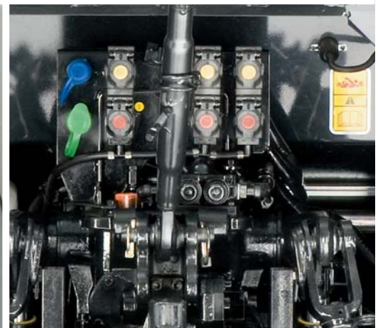
Hydraulic equipment: up to three remote valves.
