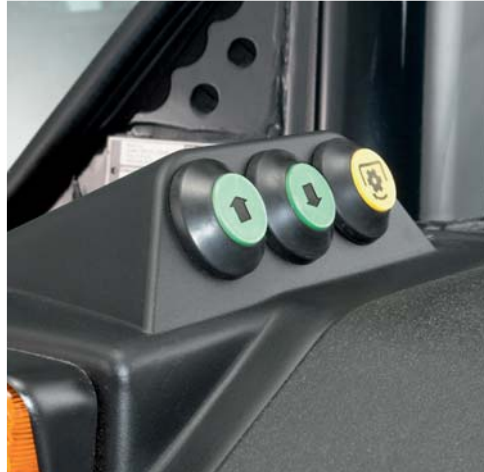
Everything to hand and in sight: the rear controls for the rear powerlift.
