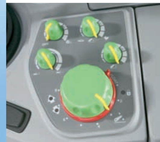
The standard EHR operating panel permits fast programming and setting adjustments.
