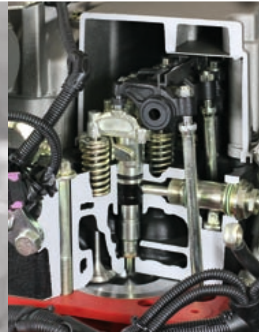
Optimum fuel combustion thanks to four valves and 6-hole injection nozzles.
