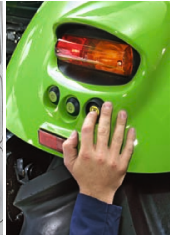
The powerlift and PTO can also be operated from the mudguard.
