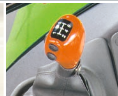
6-speed main transmission and the four-powershift stages can be conveniently operated on the gearshift lever.
