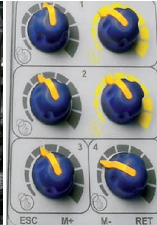
The flow rate and time are set in the armrest.
