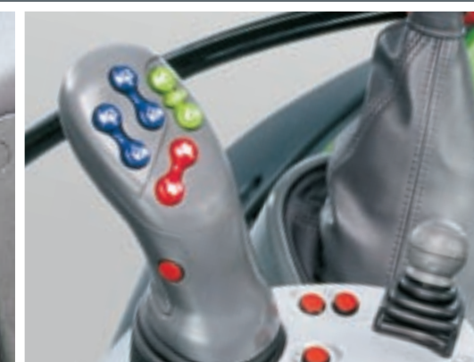
The powershift stages can also be shifted at a touch with the PowerComS operating lever.
