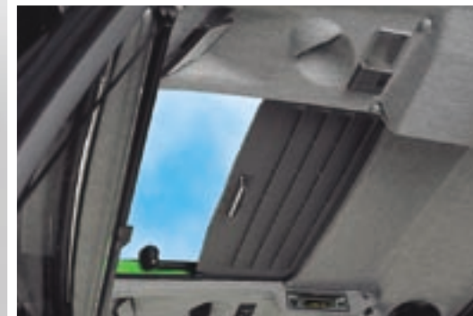
The tilting roof has a blind to enable it to be darkened.
