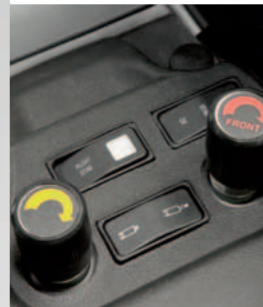
Electrohydraulic lateral stabilization and flow rate controllers for accessories.
