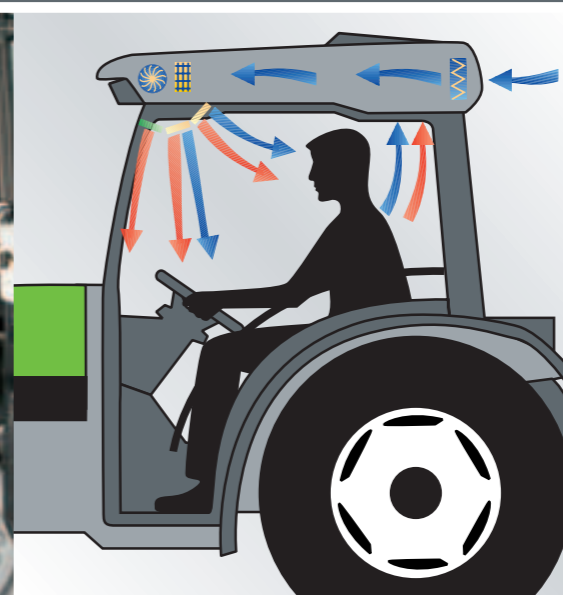
Heating, ventilation and air conditioning (upon request) are located in the cab roof.
