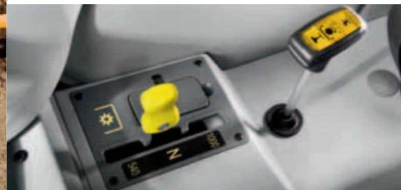
Comfortable in-cab pre-selection of four PTO speeds.
