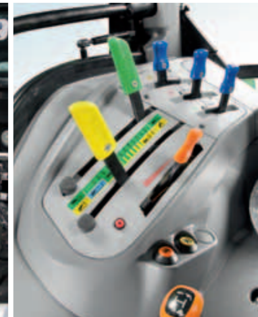
Mechanical rear lift controls.
