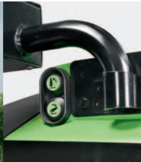
External control of electronic lift on both the rear mudguards.
