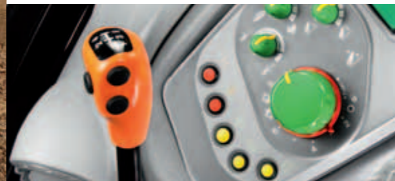
Easy to shift: The 40/40 speed Hi-Lo transmission.
