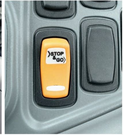
Stop & Go is activated per toggle switch.
