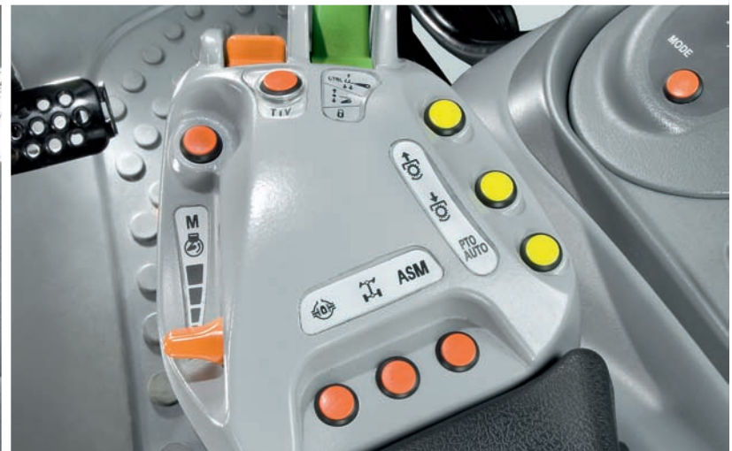
Electro-hydraulically operated PTO (push-button control).
