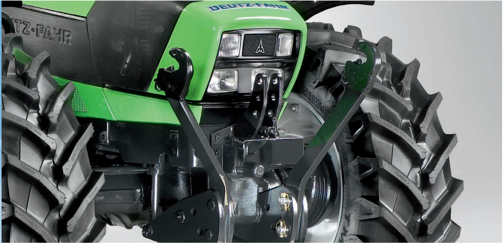
Fully integrated, powerful front hydraulics with 1.8 t lifting force.
