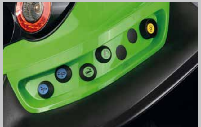
External control for auxiliary hydraulics, rear lift and PTO mounted on both sides of the tractor.
