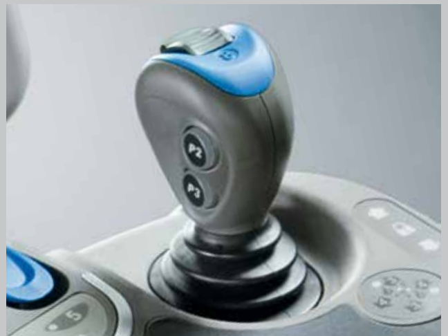
Auxiliary valves are controlled via a joystick with an integrated smart wheel.
