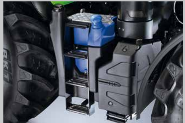
Less fuel and AdBlue consumption. 400 L diesel and 50 L AdBlue tank for long working days.
