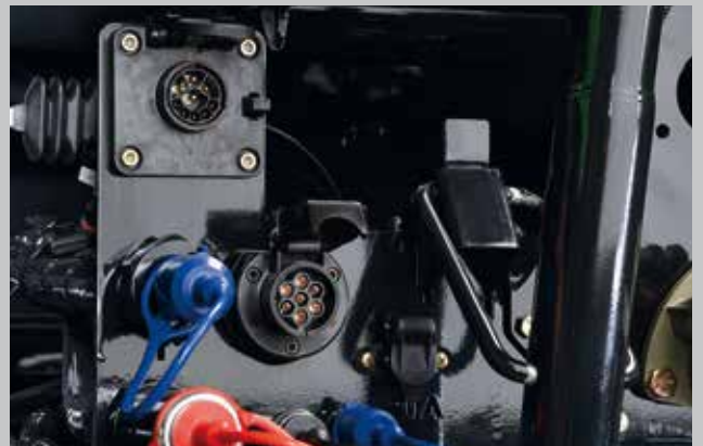
Rear mounted ISOBUS interface..
