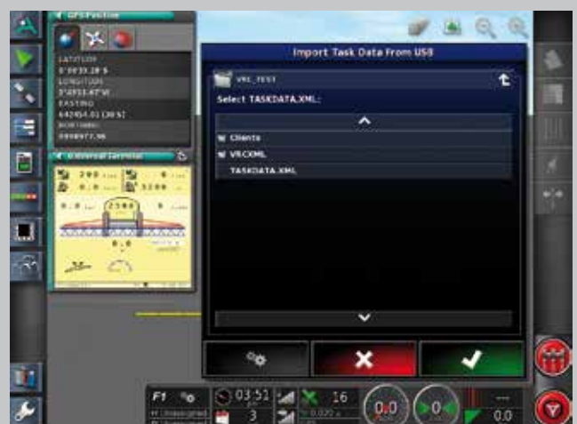
Wireless data sharing as an option and data management (ISOMXML) as standard.
