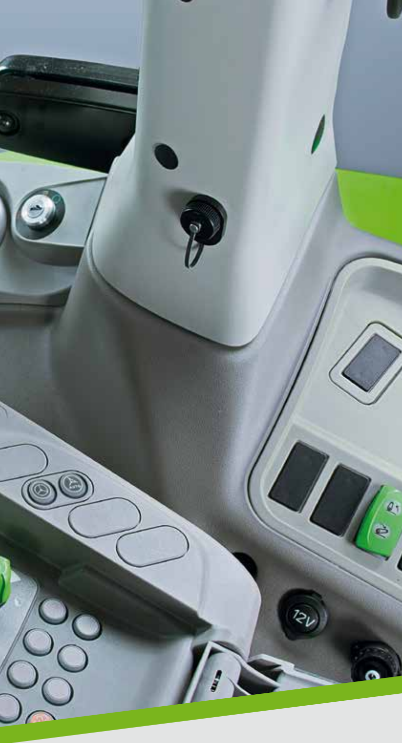
PTO controls (front/rear) are conveniently integrated in the armrest...
