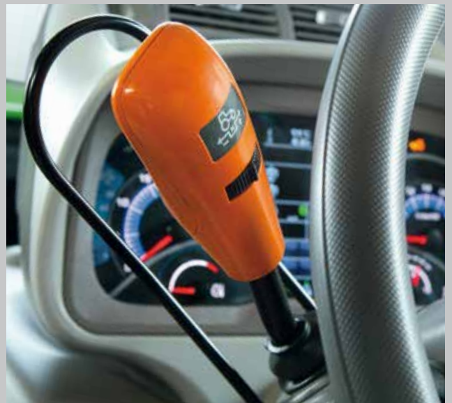
PowerShuttle with SenseShift - 5 levels of reversing sensitivity that can be easily adjusted.
