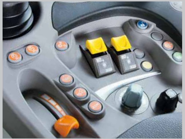
PTO controls (front/rear) are conveniently integrated in the armrest...
