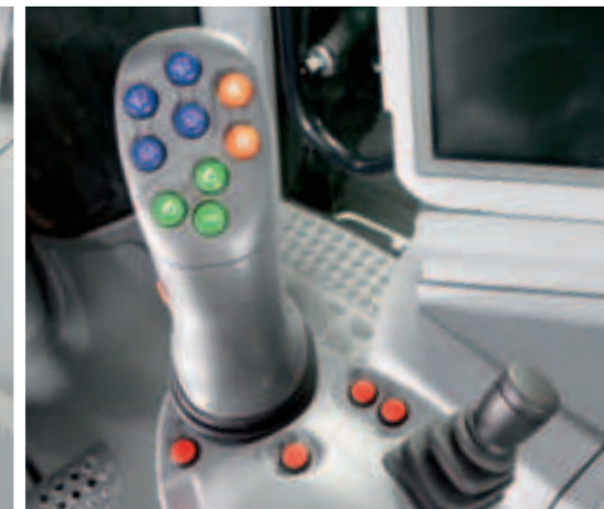
Multifunction joystick with integrated hitch controls.
