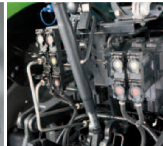
Up to 7 hydraulic spool valves with a total of 10 rear ports and 2 front ports, plus control of the front lift.
