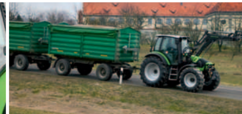
The TrailerStretch function, activated by a button in the cab, allows you to have a dual braking (transmission + brakes) in "Auto" mode.
