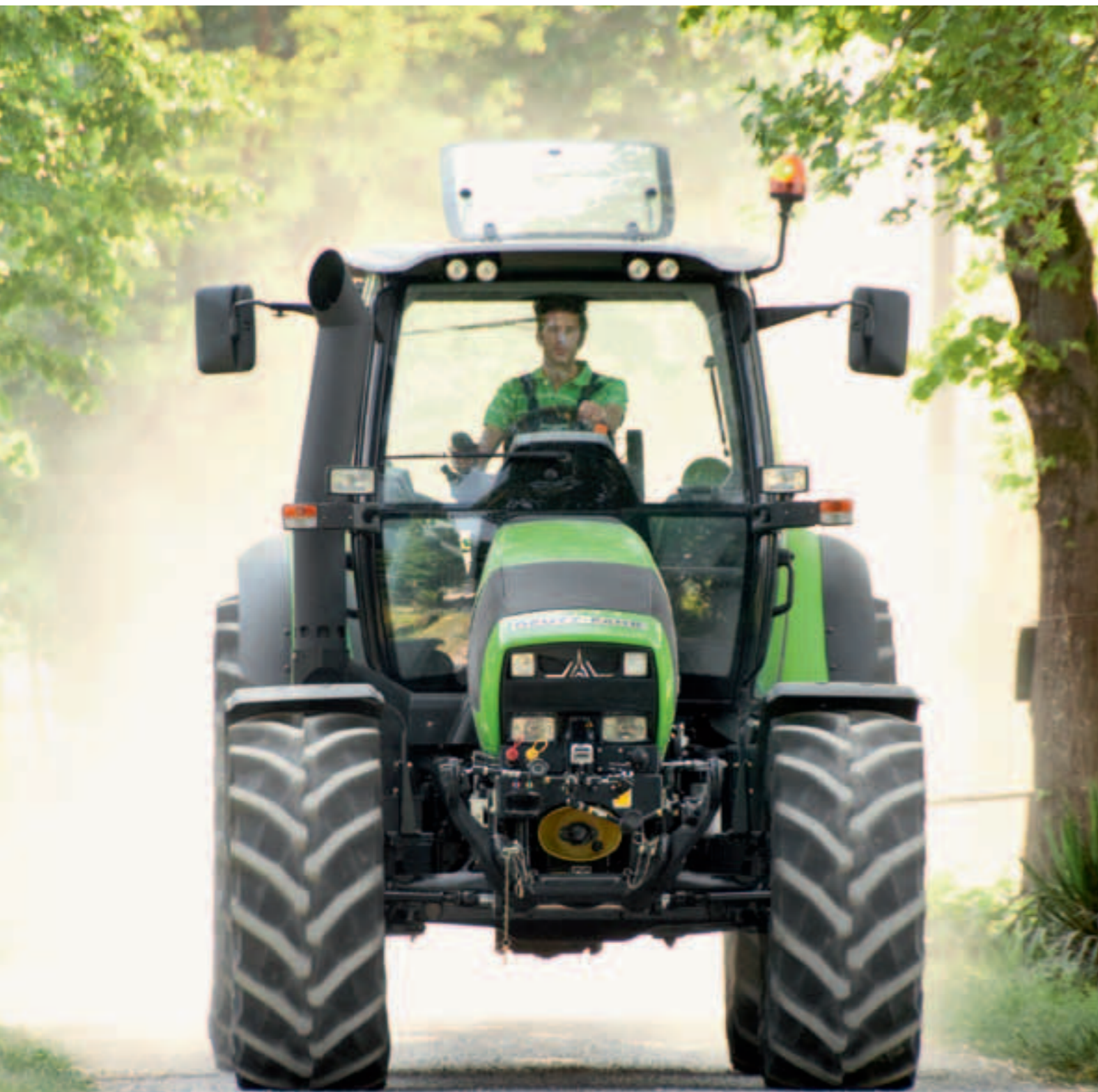
The trunnion mount creates a fulcrum coinciding with the centre line of the axle, allowing an oscillation of 22° at either end to negotiate even the roughest terrain.
