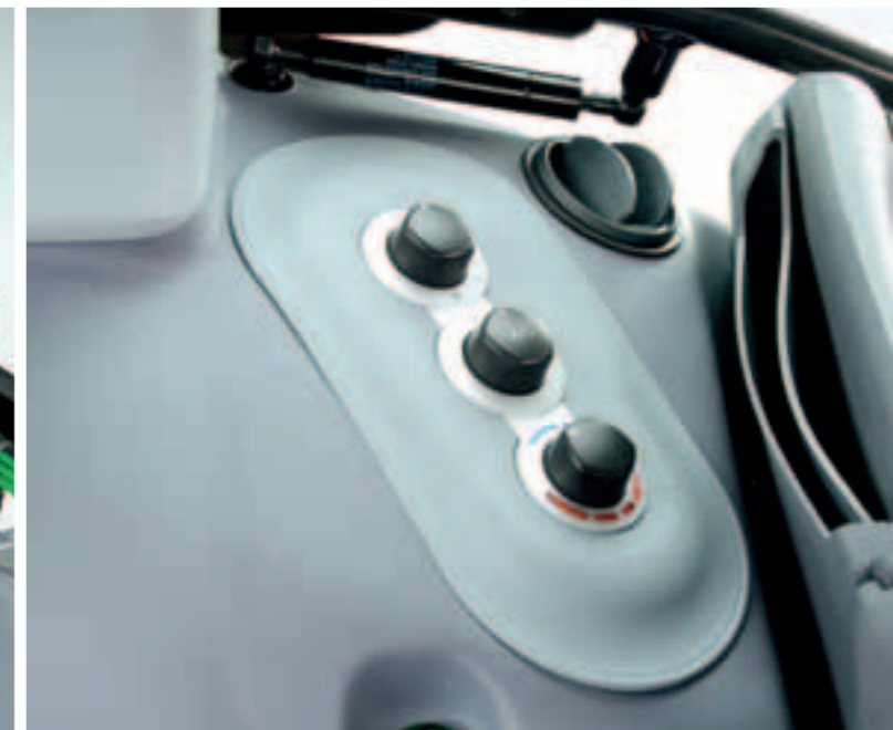
Ventilation system with a powerful installation with 4 speeds and a flow of 580 m 3 /h.
