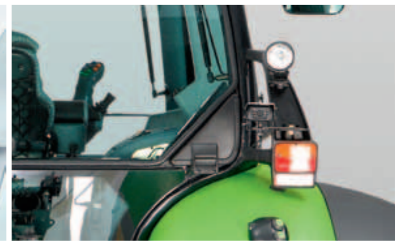
Access point for cables and Power sockets on the same side: 4-pin standard implement connector; external power socket; socket allowing transfer of data between tractor and implement.
