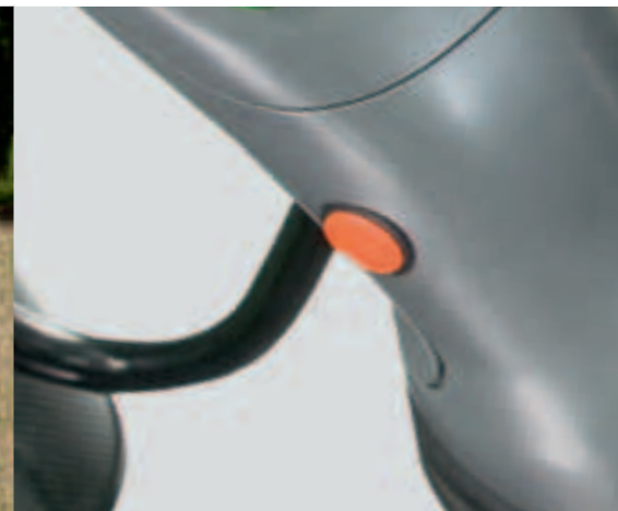
A simple pushbutton activates the programmed cruise speed.
