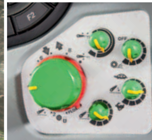
Lift movements and settings are selected from a side console and indicated by a digital display on the main instrument panel, in which the driver can view the various operating parameters.
